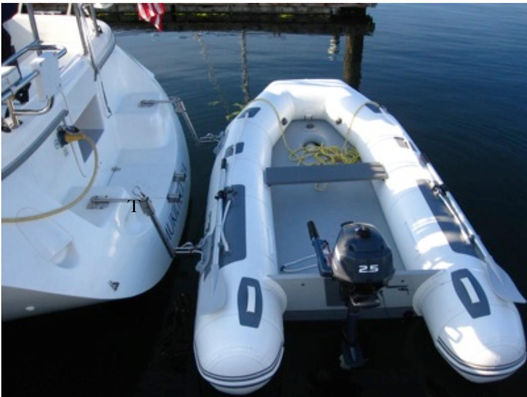
Side View of Inflatable Dinghy Snapped onto Removable Davits
