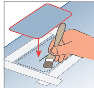
suede. Wipe the surface of the patch and the tube that is going to have the adhesive on with the P510 solvent cleaner. Allow the solvent to flash off (evaporate). If you apply the adhesive to soon it will bloom (turn slightly white) the adhesive will need to be removed and new adhesive will have to be applied.
