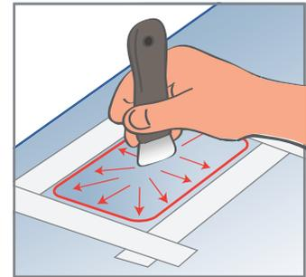
**9.** Put down the patch and rub down from the centre out with your Smoother. Check that all the edges are stuck down.
