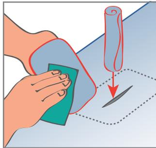
**3.** Mix half of the adhesive (2990 two part adhesive) as directed on the tin. Brush onto the surface thinly, the surface should look wet. Allow the adhesive to dry for at least 30 minutes.
